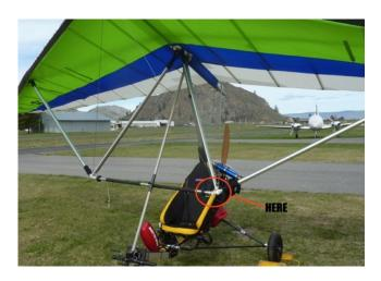
There were two types of fittings (short and long). The short ones go up inside the strut and you cannot see the cotter pin through the pin install hole. So you must take the fitting out of the strut.
