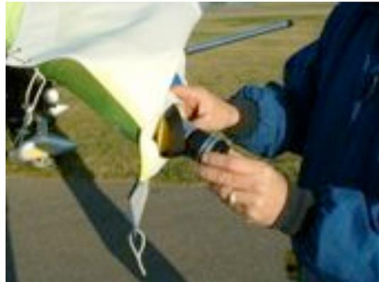
**Step 5:** Slip shim over the trim tip, and reinsert trim tip into leading edge. Shims range from 1/4” to 3/4”.
