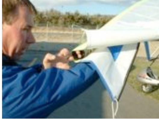
**Step 3:** Using the black strap attached to the sail, pull the yellow strap out of the groove in the trim tip. This may require removing the sail screw at the nose going into the leading edge so the sail can slide back to allow slack in the yellow strap.
