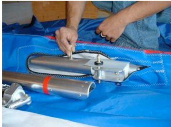
Now install the eye bolt through the X-bar channel bracket. X-bar onto the 3/8" eyebolt. To do this follow the picture. 1/4" thick plastic spacer, mylar, channel bracket, white nylon washer (between the bracket and X-bar), X-bar. On the inside of the X-bar you will have the Half moon spacer, SS finder washers, and std. washer, then the castle nut and safety.
