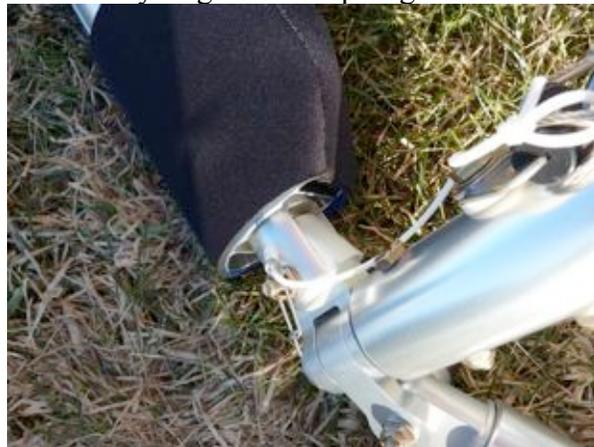
7. HOOK UP CROSSBAR MAIN CABLE Remove pull back nylon line from spring catch. Pull the line all the way back, till you can latch the cable shackle into the spring catch. Make sure the wing tip yellow webbing is in the 1" slot on the trim tip cap before tightening the wing with cable.
