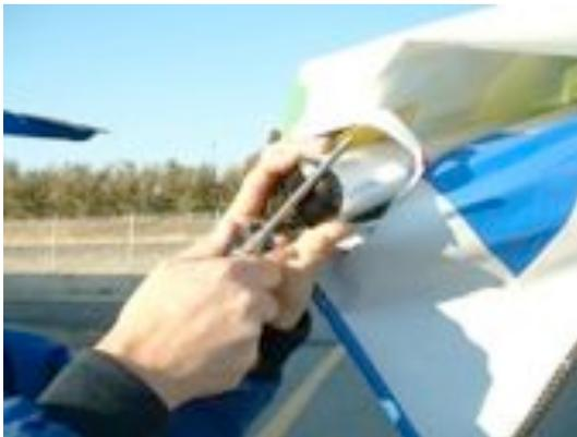
**Step 6:** Realign screws with marks on leading edge as it was when disassembled. Otherwise, wing twist will be changed as well as LE tension. Note! Tighten the screws 1-2 turns per side. Not
