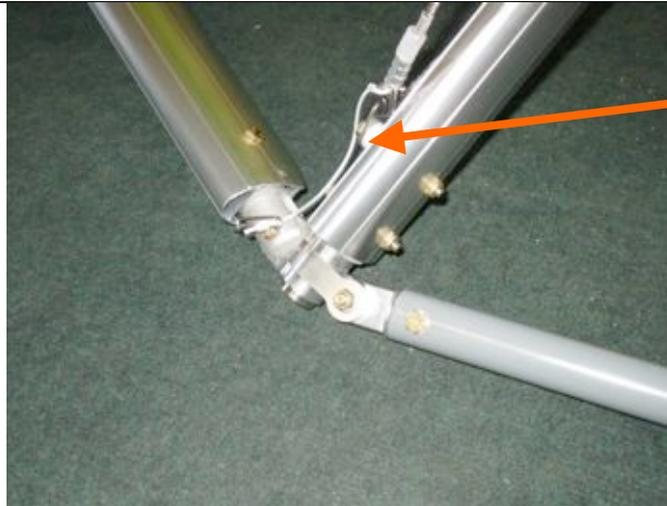
Lower front and rear cables attachment to downtube
