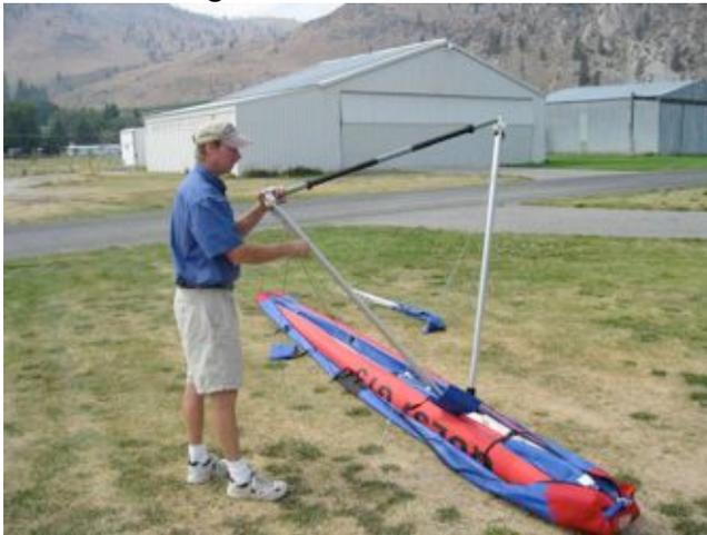
2. ROLL THE WING OVER Stand wing on the control frame (do not attach the lower front wires at this time). FIG.3
