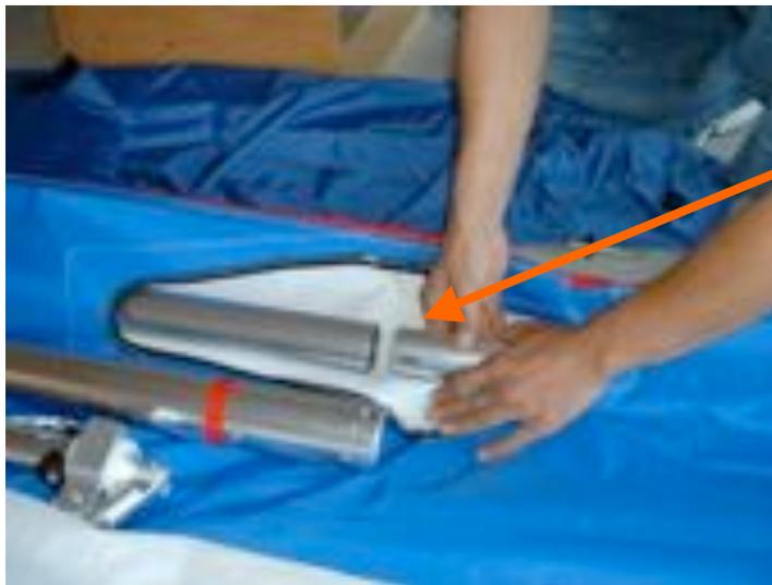
Rear section of LE separating from front section
