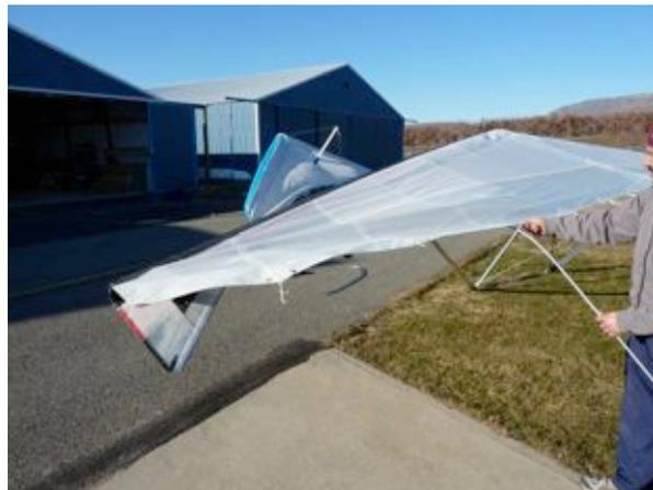
8. INSERT REMAINING RIBS Remove the tip bags and insert remaining 3 tip ribs, than lastly the straight tip struts onto LE hooks.
