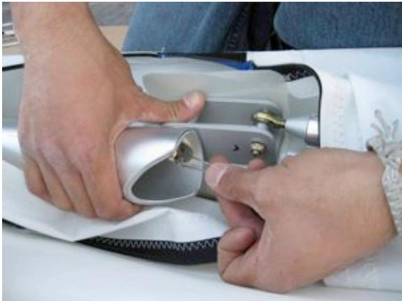
Installing the tip sail strap (yellow) over the end of the trim tip cap. Make sure that the webbing is in the 1" inch wide slot. See picture. Note: You can take the sail nose screws out of the grommet to make it easier to put the webbing over tip. After the webbing is over tip run a string from grommet to grommet and around the nose plate and tighten line to pull tension in the leading edge. Now you are ready to set up your new wing.
