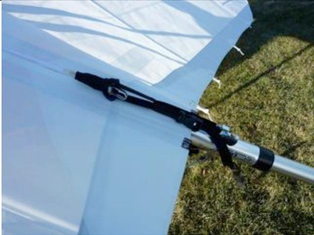
6. INSTALL STRUTS Place struts under wing on each side. There is a left and right strut and are marked. The strut also should be marked top. This is the side that has a 5/16" clevis pin. First hook up the lower end of the strut (1/4" pin) then the top. Make sure you install the safety rings and make sure that the safety rings are not sprung. FIG.7&8
