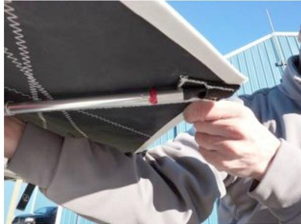
9. LOCATE SPROGS INTO POSITION (If it is light winds you can put the wing on its nose for this) Open the zipper at each sprog location, rotate the four sprogs out to center of the transversal batten. Now put the Velcro loop around the end of the sprogs. Leave Velcro loops slightly loose (apx. 1/2" gap). FIG.10&11
