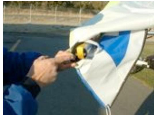
**Step 7:** Re-attach yellow strap into trim tip groove making sure strap is fully in groove.
