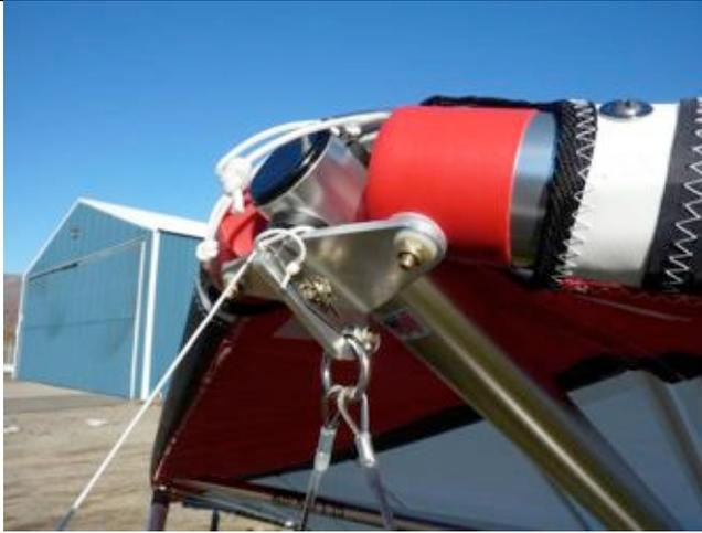
12. POSITION THE NOSE RIBS AND NOSE CONE Pull the nose down to eye level so you can put the nose rib on the 1/4" stud located front top of keel tube. With nose cone in hand start with the two top Velcro tabs and gently pull the nose cone down and around the nose plate to connect the two bottom Velcro tabs on the nose cone to its corresponding Velcro sewn on the under surface below the keel. FIG.13&14
