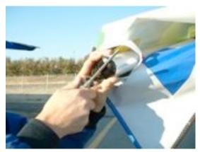
**Step 6**: Realign screws with marks on leading edge as it was when disassembled. Otherwise, wing twist will be changed as well as LE tension. Note! Tighten the screws 1 –2 turns per side. Not
