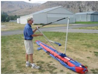
2. <u>ROLL THE WING OVER</u> Stand wing on the control frame (do not attach the lower front wires at this time). FIG.3
