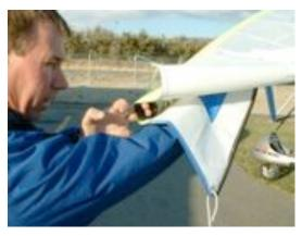
**Step 3**: Using the black strap attached to the sail, pull the yellow strap out of the groove in the trim tip. This may require removing the sail screw at the nose going into the leading edge so the sail can slide back to allow slack in the yellow strap.
