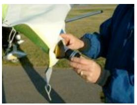
**Step 5**: Slip shim over the trip tip, and reinsert trim tip into leading edge. Shims range from 1/4" to 3/4".
