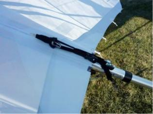
6. <u>INSTALL STRUTS</u> Place struts under wing on each side. There is a left and right strut and are marked. The strut also should be marked top. This is the side that has a 5/16" clevis pin. First hook up the lower end of the strut (1/4" pin) then the top. Make sure you install the safety rings and make sure that the safety rings are not sprung. FIG.7&8
