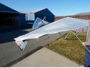
8. INSERT REMAINING RIBS Remove the tip bags and insert remaining 3 tip ribs, than lastly the straight tip struts onto LE hooks.
