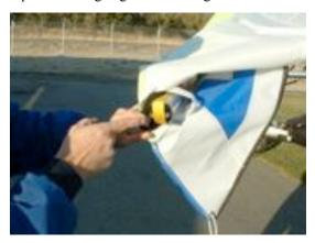
**Step 7**: Re-attach yellow strap into trim tip groove making sure strap is fully in groove.
