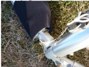
7. <u>HOOK UP CROSSBAR MAIN CABLE</u> Remove pull back nylon line from spring catch. Pull the line all the way back, till you can latch the cable shackle into the spring catch. Make sure the wing tip yellow webbing is in the 1" slot on the trim tip cap before tightening the wing with cable.
