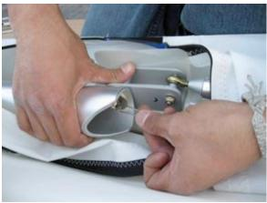
Installing the tip sail strap (yellow) over the end of the trim tip cap. Make sure that the webbing is in the 1" inch wide slot. See picture. Note: You can take the sail nose screws out of the grommet to make it easier to put the webbing over tip. After the webbing is over tip run a string from grommet to grommet and around the nose plate and tighten line to pull tension in the leading edge. Now you are ready to set up your new wing.
