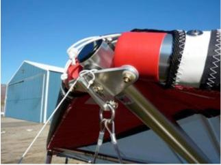
12. <u>POSITION THE NOSE RIBS AND NOSE CONE</u> Pull the nose down to eye level so you can put the nose rib on the 1/4" stud located front top of keel tube. With nose cone in hand start with the two top Velcro tabs and gently pull the nose cone down and around the nose plate to connect the two bottom Velcro tabs on the nose cone to its corresponding Velcro sewn on the under surface below the keel. FIG.13&14
