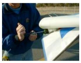
**Step 2**: Loosen both trim tip screws 4-5 full turns. Using the Philips screwdriver, "pop" the screws in with the heel of your hand to loosen the trip tip. (For more detail on how the trim tip works, see next section on **Wing Twist**.)
