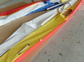
Turn the sprogs so they point towards the tip. Slide the rear section into the front section until the hole lines up. Install bolt from the bottom up, wrap the mylar protector around the LE and put over the bolt, now thread the nut on over the mylar. Tighten snug. Do not over tighten or you
