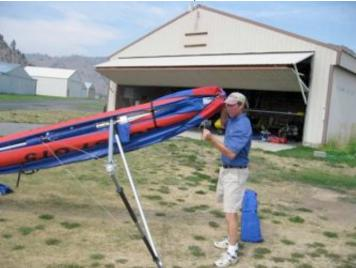
3. <u>REMOVE BAG. SPREAD WINGS</u> Ensure that the keel stand "stinger" is in place. Carefully walk each wing out to 3/4 of it's own approximate flying position. Leave enough slack in the sail so that during the next step the ribs may slide in with minimal resistance. FIG.4
