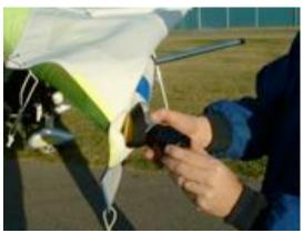
Step 4: Slide the trip tip out of the end of the leading edge.
